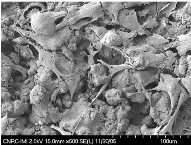
Fig. 17 Osteoblast cell culture (7 day-incubation) on the surface of an APS conventional HA coating
